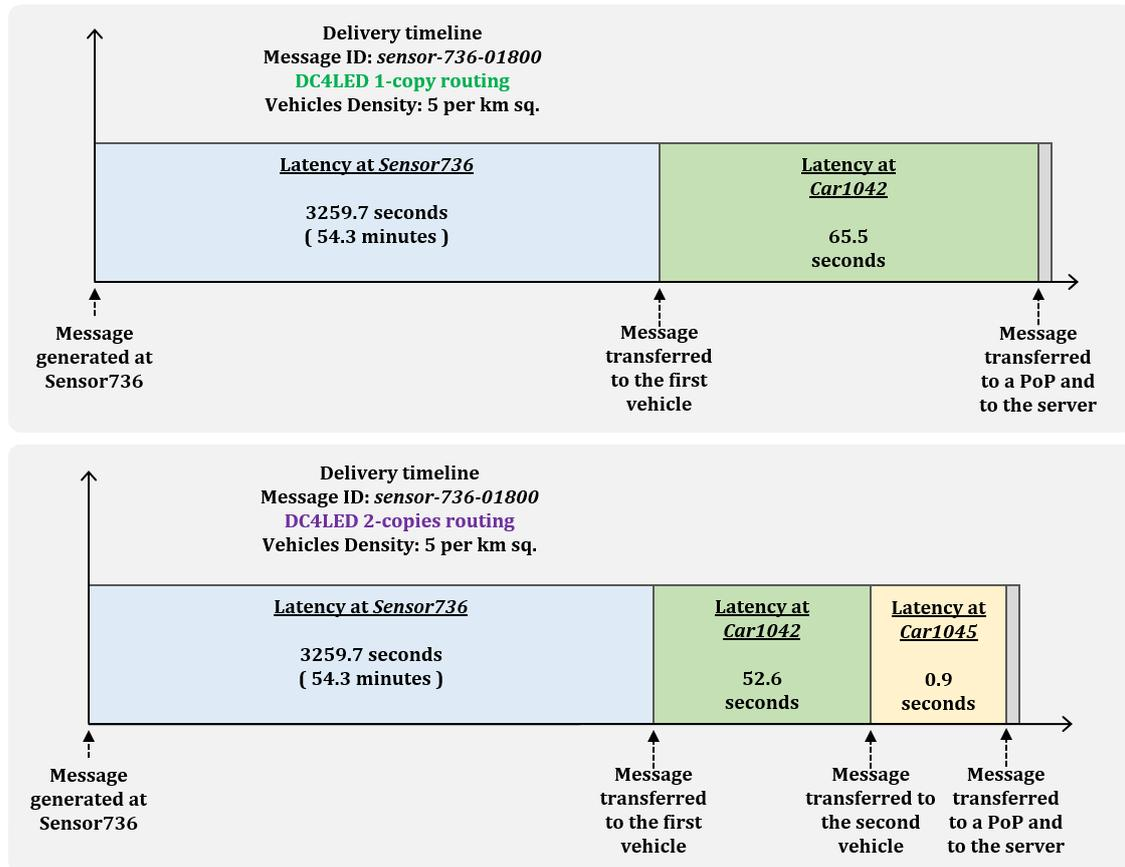
Figure 7.6 – An Example of Messages Delivery Timeline for The DC4LEDx 1-Copy and 2-Copies Routing at Vehicles Density of 5 per km<sup>2</sup>
