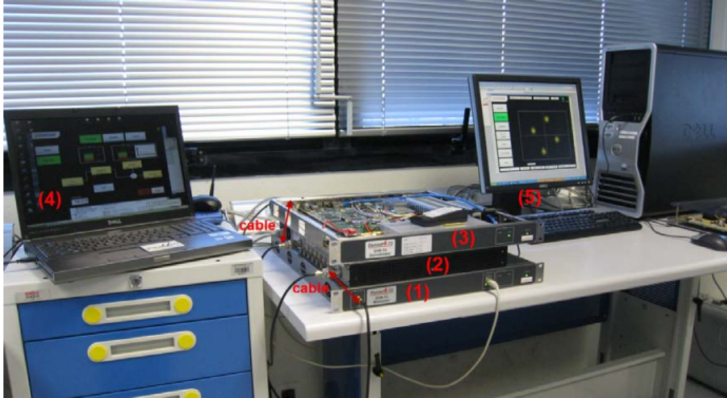
Figure 1.2: DVB-T2 transmitter, channel emulator and receiver of Teamcast integrating proposed BICM receiver demonstrated at IBC 2010.
