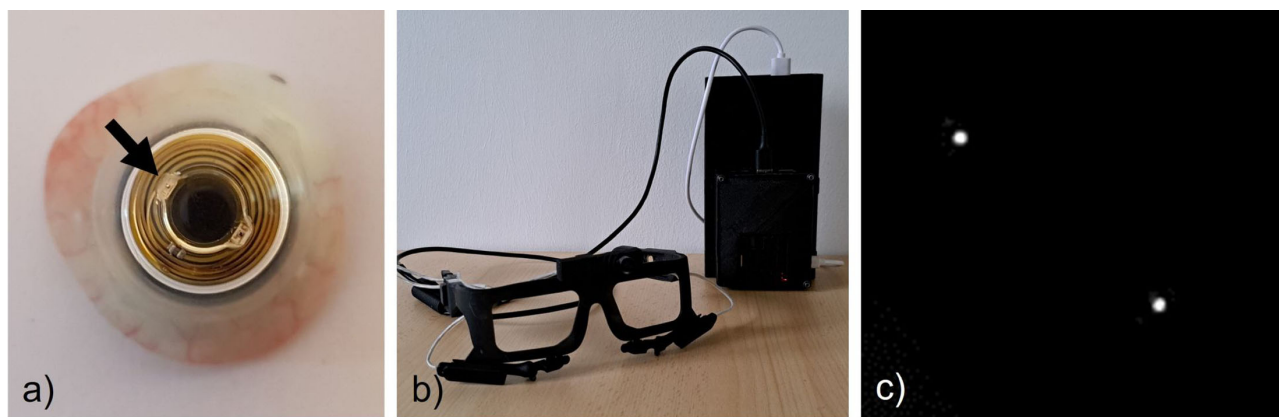
Figure 1. CLP elements. (a) The contact lens on an ocular prosthesis (the black arrow shows the position of one VCSEL). (b) The eyewear with the primary antenna inside and the Pupil Core camera, Raspberry Pi, and its associated battery. (c) Example of an eye camera capture of the VCSEL spots.
