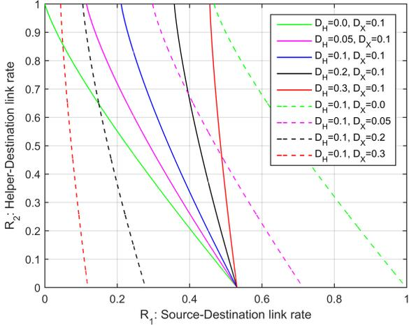
Fig. 4. Admissible RD region for the stage 2 with different distortions  $D_H$  at Helper, and for different distortion requirements  $D_X$  at Destination.
