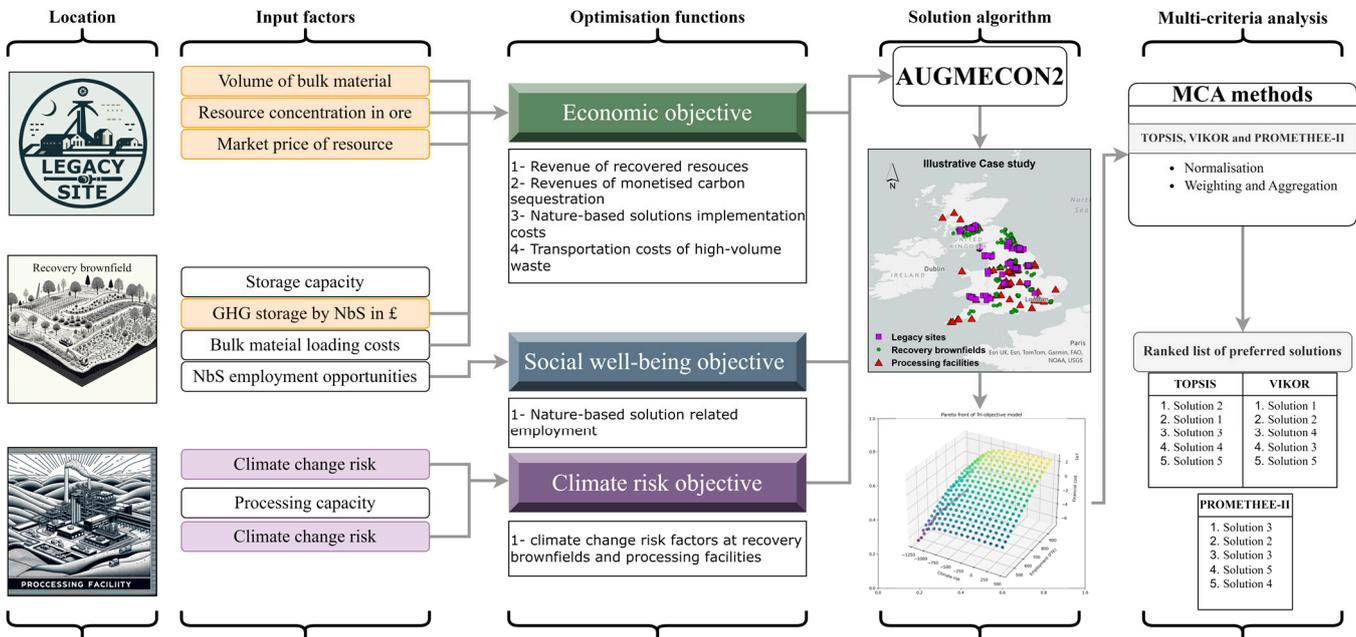
**Figure 1.** Network schematic of the nature-based secondary resource recovery. The orange-coloured input factors are subject to sensitivity analysis of the deterministic model, whereas the purple-coloured input factors are part of the robust optimisation approach.
