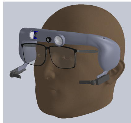
Figure 3. Illustration of the headband on a face. The headband was designed so that it could be used by spectacle wearers. We can distinguish the two cameras of the eye tracking module which are under the eyes, slightly in front of the glasses.
