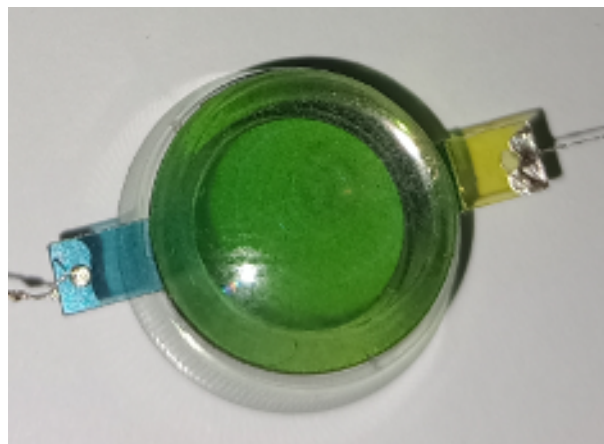
Figure 6: Integration of the electrochromic display in a scleral contact lens
