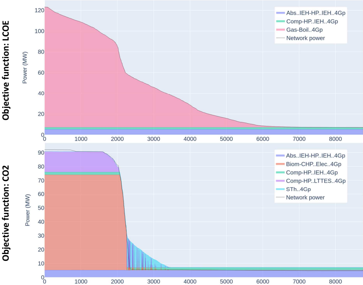
Figure 5: Duration curve of the thermal power carried by the 4GDHnetwork. Scenario (SE-HR) for the architecture NN_4G_DC.
