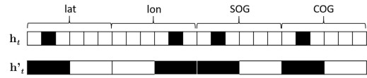
FIGURE 3. Example of multi-resolution “four-hot” vectors for AIS data: The model uses the fine-resolution vector h_t in the embedding module (see Fig.2), while the loss function uses both h_t and a coarse-resolution h'_t .
