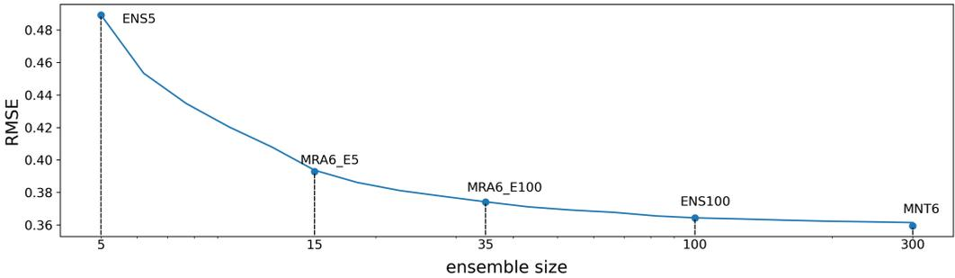
**FIGURE 12** RMSE of the ensemble Kalman filter as a function of the ensemble size. The dots show the RMSE of the different experiments shown in Fig. 11 but plotted over the line to relate the performance of the machine learning technique to the ensemble size of the ensemble Kalman filter.
