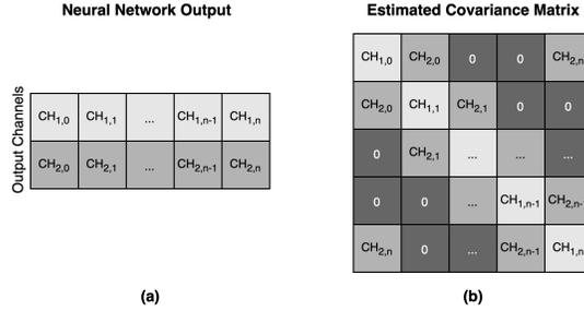
**FIGURE 3** The output of the network is shown in panel (a), the  $i^{th}$  element of channel 0 is the variance corresponding to the  $i^{th}$  state variable. The  $d^{th}$  channel corresponds to the covariance between the state variables separated by a distance  $d$  as shown in panel (b). Covariance values not represented with the ANN output are assumed to be zero.
