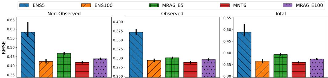
**FIGURE 11** RMSE of different assimilation experiments where ENS100 and ENS5 correspond to the ensemble Kalman filter performance for a 100 and 5 ensemble respectively. MNT6 corresponds to the performance of a neural network trained with the ground truth, MRA6\_E5 is a network trained with the 5-member ensemble dataset and MRA6\_E100 is the network trained with a 100-member ensemble dataset.
