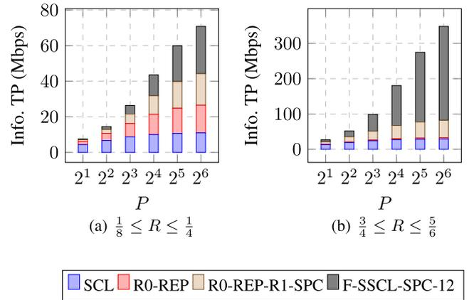
**FIGURE 11.** Maximum information throughput of SCL decoder and various polar code decoders with different pruning techniques as a function of  $P$ . Low and high code rates are considered with  $N = 1024$ .
