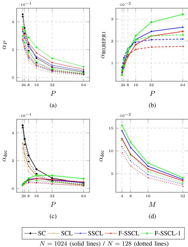
**FIGURE 13.** Average utilization rates of several SC-based decoders of length  $N = 1024$  (solid lines) and  $N = 128$  (dotted lines): (a)  $\alpha_P(P)$ , (b)  $\alpha_{SND}(P)$ , (c)  $\alpha_{dec}(P)$ , (d)  $\alpha_{dec}(M)$ .
