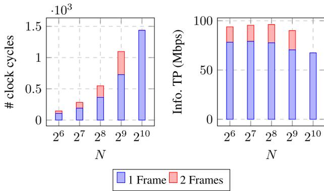
FIGURE 15. Latency and throughput as a function of code length  $N$  for a multi-frame SSCL decoder.
