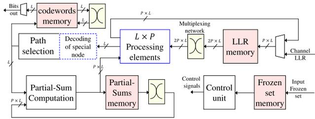
FIGURE 2. Semi-parallel architecture model for SCL decoders.
