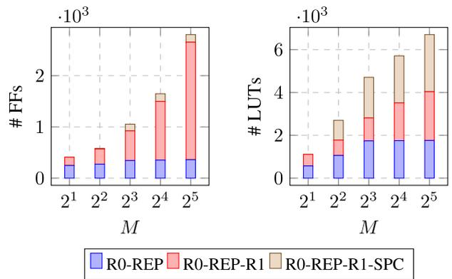
**FIGURE 9.** Number of FFs and LUTs required by SNLD to decode special nodes R0, REP, R1 and SPC when considering the second approach with accumulator registers to reduce the number of adders, comparators and XOR gates.
