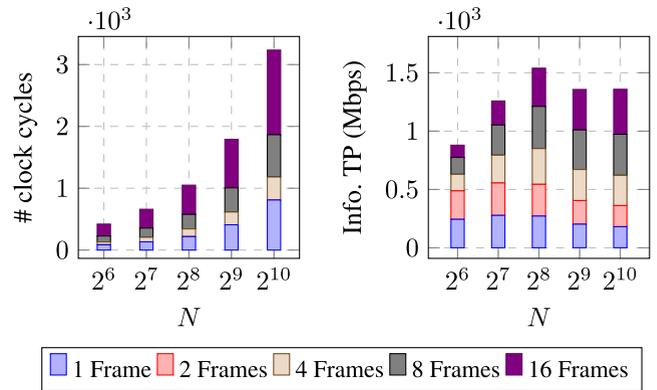
FIGURE 16. Latency and throughput as a function of code length  $N$  for a multi-frame Fast-SSCL-1 decoder.
