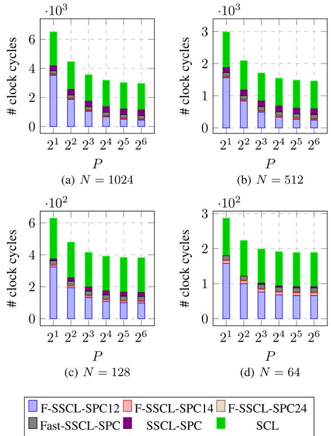
FIGURE 3. Number of clock cycles required to decode one polar code frame for a varying number of PEs. Worst-case latency is reported while varying the value of  $R$ . Results are given for SCL and five related variants of simplified algorithms.
