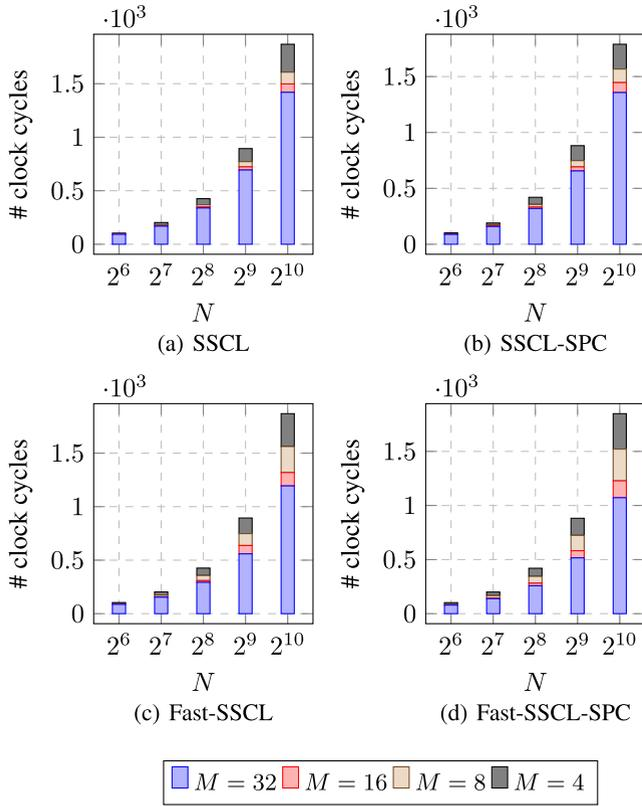
**FIGURE 4.** Number of clock cycles required to decode one polar code frame as  $N$  varies from 64 to 1024. Average latency is reported while varying the value of  $R$ . Results are provided for various values of  $M$  and are reported for four different algorithms.
