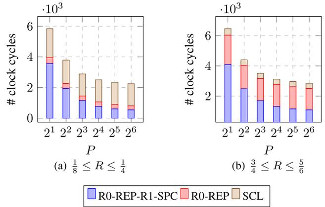
**FIGURE 5.** Number of clock cycles required to decode one polar code frame for a varying number of PEs and different pruning techniques. Average latency is reported and results are given for low and high code rates.
