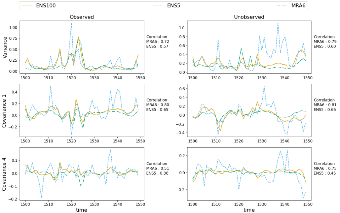
FIGURE 5 Time evolution of selected covariance matrix elements over 100 consecutive time steps starting at the 1500 cycle of the testing set. The panels, from top to bottom, show respectively the first elements of the first column of the covariance matrix. Left panels show covariance matrix elements of an odd row (centered at observed variables), while right panels shows covariance matrix elements of an even row (centered at an unobserved variable). The correlation coefficient computed over 15.000 assimilation cycles, between ENS5 and MRA6 with respect to ENS100 are shown to the right of each panel.
