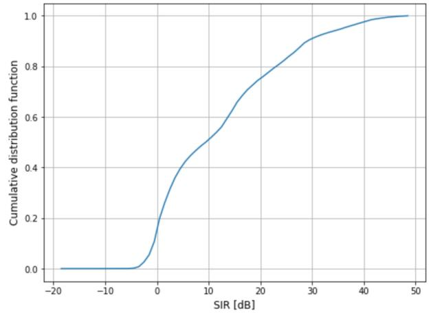
Fig. 15: Cumulative distribution function of the SIR
