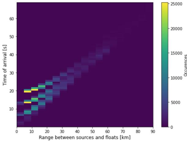
Fig. 11: ToA distribution as a function of distance
