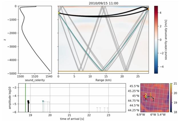
Fig. 3: Example of an oceano-acoustic simulation snapshot
