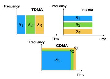
Fig. 6: Scheme of the method of spectrum resource sharing
