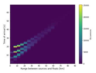
Fig. 11: ToA distribution as a function of distance
