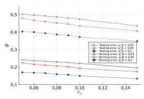
Figure 3: Error exponents as functions of  $p_g$ , for various values of  $p_b$  and for  $\bar{p}_G=0.3$ ,  $\bar{p}_B=0.5$ , g=0.001, b=0.002, p=0.2,  $\delta=0.001$ .
