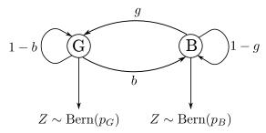
Figure 1: Gilbert-Elliot model for the correlation noise Z under hypothesis  $\mathcal{H}_0$ . Under hypothesis  $\mathcal{H}_1$ , the crossover probabilities become  $\overline{p}_G$  and  $\overline{p}_B$ , while the parameters g and b remain the same.
