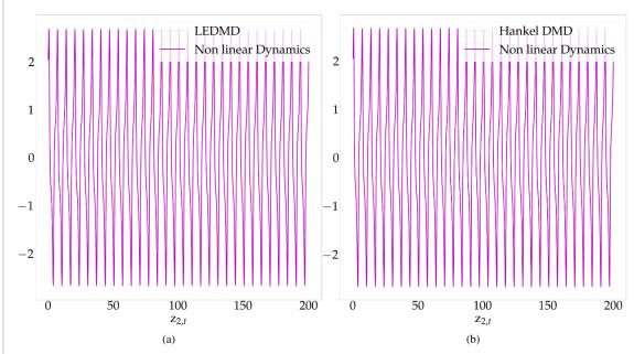
Figure 9. Time series of the data-driven Koopman models with respect to the true non-linear oscillator. (a) Proposed LEDMD model; (b) Hankel-DMD model.
