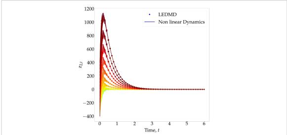
**Figure 4.** Simulation of the non-linear dynamical model (42) using the LEDMD model constructed on partial observations of the state variables. The colors correspond to simulations from different initial conditions. The lines correspond to the non-linear dynamics of  $z_{2,t}$  and the dots represent the LEDMD simulation. Even with partial measurements of the non-linear dynamics (42), the proposed framework perfectly matches the ground truth.
