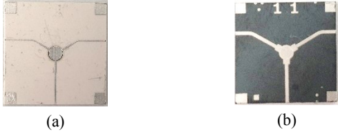
Fig. 4. Manufactured circulators: (a) Garnet1900-based; (b) Spinel3800-based
