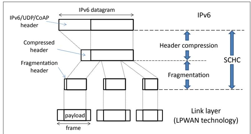
FIGURE 2. SCHC functionality overview: header compression and fragmentation.
