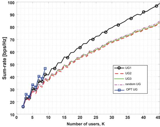
Fig. 4: The sum-rate performance of different MB-NOMA UG algorithms versus the number of users for the SB-MB-NOMA-RRFC scheme. The sum-rate is averaged over 5,000 trials.
