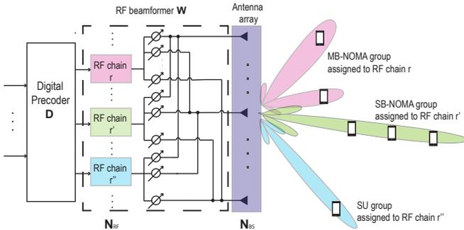
Fig. 1: Joint single- and multi-beam MIMO-NOMA scheme.
