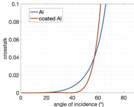
**Fig. 2.** Influence of the oblique incidence on the crosstalk ratio for a noncoated aluminium surface (blue line) and an aluminium surface coated with a layer of index  $n = 1.4$  and thickness  $e = 112$  nm for  $\lambda = 550$  nm (red line)
