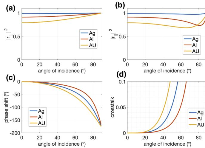
**Fig. 1.** Comparison of different metals for (a) perpendicular and (b) parallel Fresnel coefficients, (c) phase shift and (d) crosstalk ratio as a function on the angle of incidence, for  $\lambda = 550$  nm.
