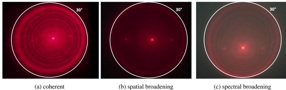
**Fig. 15.** Screen sample with random size and position of Lambertian kernels illuminated with a collimated laser beam on a 1 mm wide surface (a), a collimated laser beam on a 3 mm wide surface (b) and a weakly converging beam from a typical red source from a BenQ projector ( $\Delta\lambda \approx 120 \text{ nm}$ ) (c)
