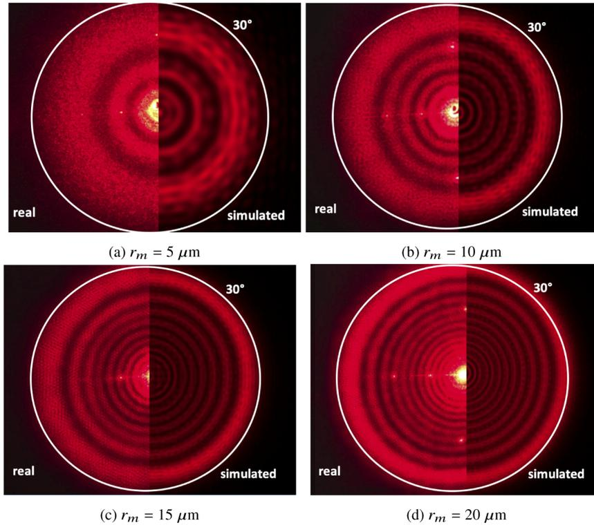
**Fig. 12.** Comparison between the experimental diffraction patterns (left) and simulated diffraction patterns (right) for  $r_m = 5 \mu\text{m}$  (a),  $r_m = 10 \mu\text{m}$  (b),  $r_m = 15 \mu\text{m}$  (c) and  $r_m = 20 \mu\text{m}$  (d)
