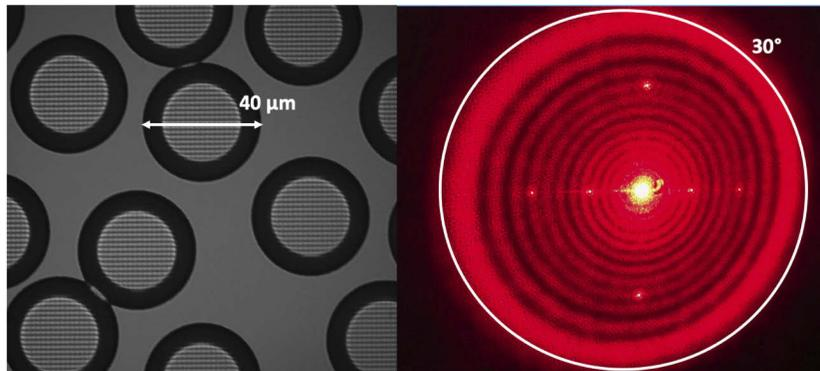
(a) randomly tiled kernels ( $r_m = 20 \mu\text{m}$ ) observed on an optical microscope
