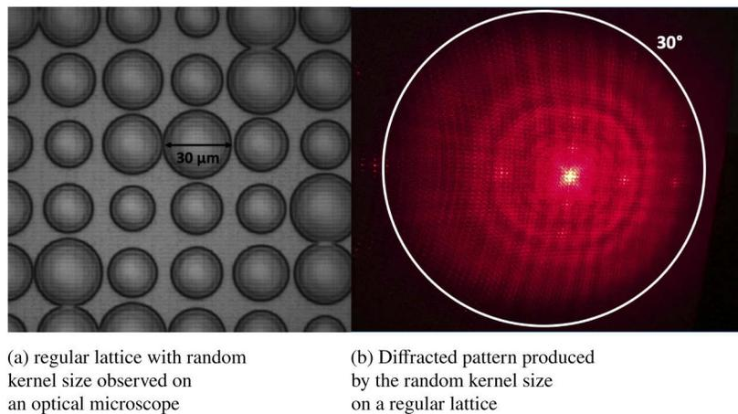
(a) regular lattice with random kernel size observed on an optical microscope (b) Diffracted pattern produced by the random kernel size on a regular lattice
