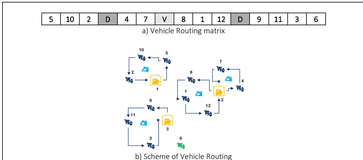
Figure 4. Vehicle Routing Representation
