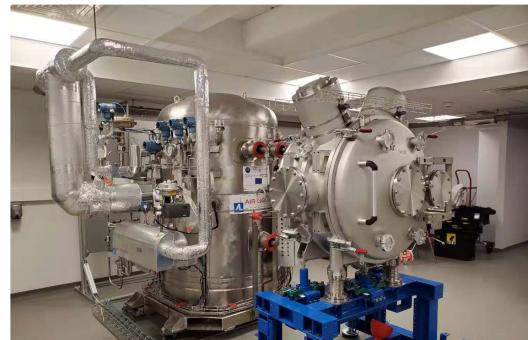
Fig. 2. Installation of the XEMIS2 cryostat and the cryogenic subsystem ReStoX in a small animal medical imaging center CIMA at Nantes Centre Hospitalier Universitaire (CHU).
