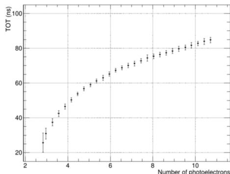
Fig. 6. Correlation between the number of photoelectrons (pe) and the Time-Over-Threshold (TOT) with a threshold of 2 pe.
