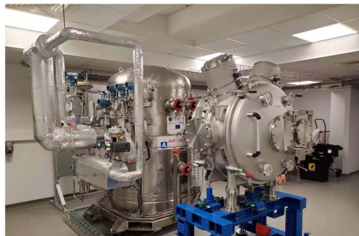
Fig. 2. Installation of the XEMIS2 cryostat and the cryogenic subsystem ReStoX in a small animal medical imaging center CIMA at Nantes Centre Hospitalier Universitaire (CHU).
