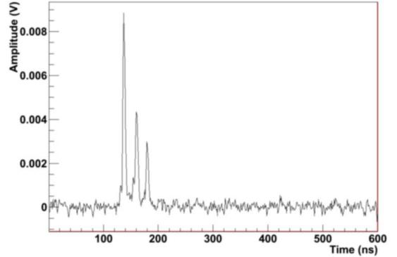
Fig. 3. Example of output signal of the photomultiplier tube (PMT).
