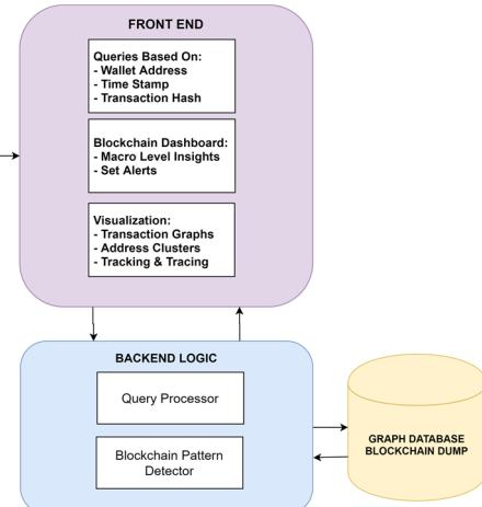
Fig. 3: Overview of the Blockchain Analysis Tool
