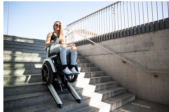
Fig. 1: Example platform and application scope: Scewo Bro wheelchair traversing a staircase ( https://scewo.ch/en/bro/ ).
