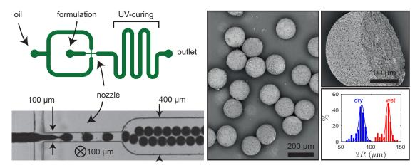
**Figure 8. Left**: schematic principle view of the microfluidic setup used to produced particles. **Right**: SEM views of the particles after calcite dissolution and drying, and histogram of size reduction after drying.
