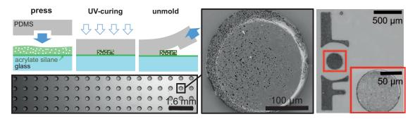
**Figure 9.** Sketch of the soft embossing process with a PDMS stamp designed with micro-cavities, here cylindrical cavities on a square lattice. The stamp squeezes the formulation in the cavities and may lead to well defined patterns on a substrate after UV-curing and acidic treatment. The pictures show a small part of the patterned substrate and a magnification on one cylinder, and also the logo of our lab (LOF) soft-embossed the same way.
