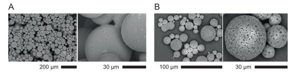
**Figure 7.** Batch particles produced by manual emulsification followed by UV-curing. (**A**) low density of calcite (before and after removal of calcite, left and right respectively where the calcite particles show as bright spots); (**B**) high density of calcite after its removal.
