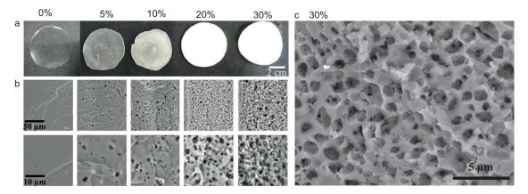
**Figure 4.** (a) monoliths prepared with volume fractions of calcite between 0 and 0.3, observed here after photo-polymerization, calcite removal by acidic dissolution, and drying; (b) SEM views of cut samples of the same monoliths for two magnifications; (c) close up of a porous polymer with 0.3 porosity.
