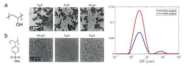
**Figure 1. Left**: (a) chemical formula of poly(vinyl alcohol) (PVA) and pictures of formulations containing calcite and PVA (concentration given above the image); (b) chemical formula of poly(sodium 4-styrenesulfonate) (PSS) and pictures of formulations containing calcite and PSS. In both cases, the mass fraction of calcite is 2%. **Right**: size distribution of  $CaCO_3$  powders in water with PSS or PVA (2% w/w of particles in a 2 g·L<sup>-1</sup> PVA or PSS solution).
