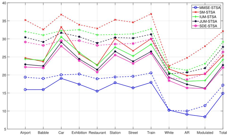
**FIGURE 3.** SNRI with various noise types for all STSA-based methods with and without the reference noise power spectrum. Dashed lines correspond to measurements obtained with reference noise power spectrum. The solid lines represent the performance measurements returned by the algorithms combined to B-E-DATE for noise spectrum estimation.
