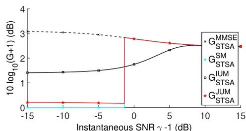
**FIGURE 1.** Attenuation curves of all joint detection/estimations in comparison with the standard MMSE-STSA method at a priori SNR level  $\xi = 5$  dB. The detector thresholds were calculated with  $\alpha = 0.05$  and  $\beta = -25$  dB.
