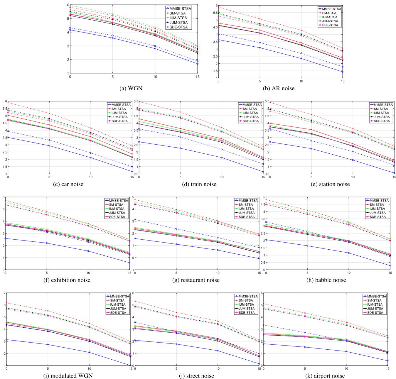
**FIGURE 2.** Speech quality evaluation by SSNR improvement after speech denoising using STSA-based methods for stationary, slowly-changing, speech-like and fast-changing non-stationary noise. Performance measurements of MMSE-STSA, SM-STSA, IUM-STSA, JUM-STSA and SDE-STSA with reference noise power spectrum are represented by dashed solid lines. The solid lines correspond to the performance measurements obtained by these same algorithms when the B-E-DATE is used to estimate the noise spectrum.
