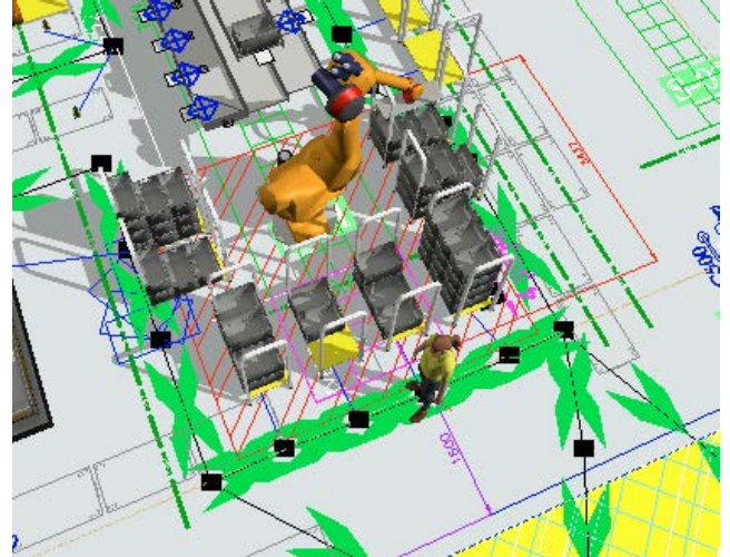
Fig. 2. Automatic loading module simulated using Flexsim.
