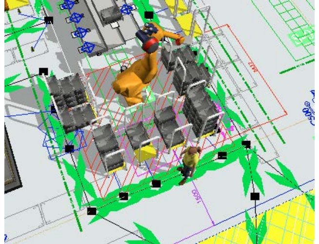
Fig. 2. Automatic loading module simulated using Flexsim.
