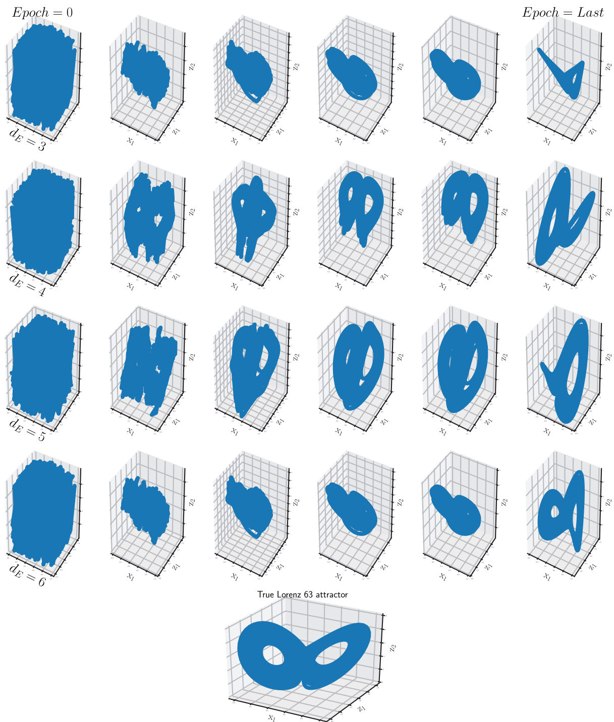
FIG. 3. Evolution of the learned latent space. Starting from a random initialization of the augmented states \mathbf{y}_i , the latent space is optimized according to the minimization of Eq. (6) to form a limit-cycle similar to the true Lorenz 63 attractor. We depict three-dimensional projections of the learned latent space for the proposed model with different embedding dimensions from d_E = 3 to d_E = 6 .
