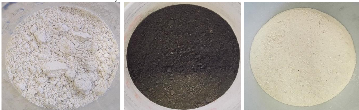
Figure 1. Images of Catalyst (A) Before Experiment (B) Residue after Experiment (C) After Regeneration
