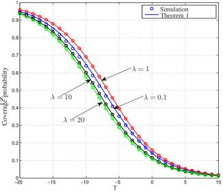
Fig. 2. Coverage probability from both Theorem 1 and simulation results.  $\alpha_{los}=2,~\alpha_{nlos}=4,~R_{los}=1{\rm m}$  and  $R_{nlos}=10{\rm m}$ .
