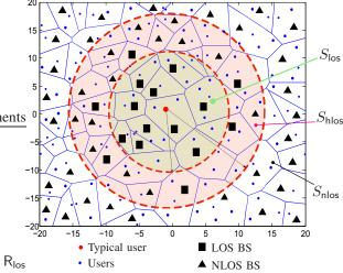
Fig. 1.  $S_{los}$  and  $S_{nlos}$  regions contain only LOS and NLOS BSs respectively, while  $S_{\text{hlos}}$  contains a mixture of the two with probability  $p(r) = 1 \cdot \frac{r - R_{\text{los}}}{R_{\text{nlos}} - R_{\text{los}}}$  for LOS BSs and  $1 - p(r) = \frac{r - R_{\text{los}}}{R_{\text{nlos}} - R_{\text{los}}}$  for NLOS BSs.
