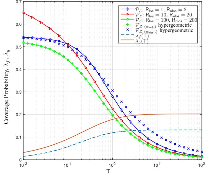
Fig. 6. Coverage probability scaling with network density  $\lambda$  for  $\mathcal{L}$  and  $\mathcal{L}_2$  path-loss models.  $R_{\text{los}} = 1\text{m}$  and  $R_{\text{nlos}} = 10\text{m}$  and path-loss exponents  $\alpha_{\text{los}} = 2$  and  $\alpha_{\text{nlos}} = 4$ .
