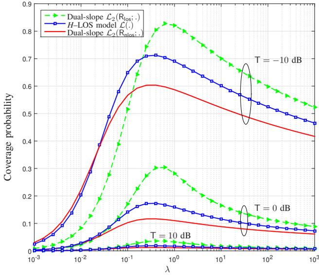
Fig. 4. Coverage probability scaling with  $\lambda$  under  $\mathcal{L}$  and  $\mathcal{L}_2$  path-loss models,  $R_{\text{los}} = 1\text{m}$  and  $R_{\text{nlos}} = 10\text{m}$ ,  $\alpha_{\text{los}} = 2$  and  $\alpha_{\text{nlos}} = 4$ .
