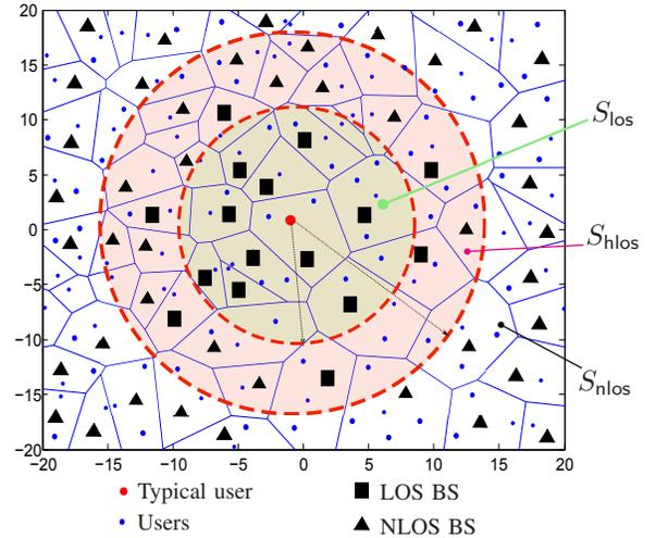
Fig. 1.  $S_{\text{los}}$  and  $S_{\text{nlos}}$  regions contain only LOS and NLOS BSs respectively, while  $S_{\text{hlos}}$  contains a mixture of the two with probability  $p(r) = 1 - \frac{r - R_{\text{los}}}{R_{\text{nlos}} - R_{\text{los}}}$  for LOS BSs and  $1 - p(r) = \frac{r - R_{\text{los}}}{R_{\text{nlos}} - R_{\text{los}}}$  for NLOS BSs.
