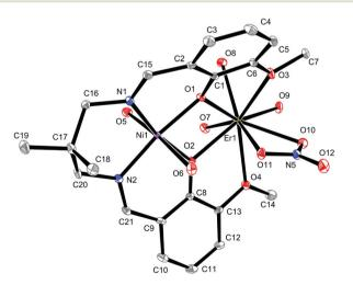
**Fig. 1** Plot of complex **1** with ellipsoids drawn at the 30% probability level with partial atom numbering and H atoms omitted for clarity. Selected bond lengths (Å): Ni–N1 2.001(4), Ni–N2 2.019(3), Ni–O1 2.025(3), Ni–O2 1.999(3), Ni–O5 2.089(3), Ni–O6 2.209(3), Er–O1 2.291(3), Er–O2 2.301(3), Er–O3 2.485(3), Er–O4 2.536(3), Er–O7 2.323(3), Er–O8 2.373(3), Er–O9 2.304(3), Er–O10 2.522(3), Er–O11 2.493(3), Ni…Er 3.4632(8) Å.
