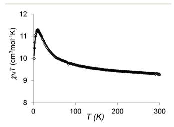
Fig. 5 Temperature dependence of the  $\chi_{\rm M}T$  product for complex 2 at 0.1 T applied field. The solid line corresponds to the best data fit (see the text).
