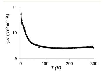
Fig. 8 Temperature dependence of the  $\chi_{\rm M}T$  product for complex 7 at 0.1 T applied field. The solid line corresponds to the best data fit (see the text).
