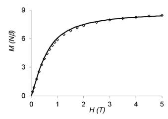
Fig. 6 Field dependence of magnetization for complex 2. The solid line corresponds to the best data fit (see the text).
