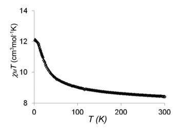
Fig. 10 Temperature dependence of the  $\chi_{\rm M}T$  product for complex 10 at 0.1 T applied field. The solid line corresponds to the best data fit (see the text).
