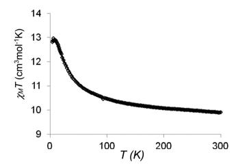
Fig. 9 Temperature dependence of the  $\chi_{\rm M}T$  product for complex 9 at 0.1 T applied field. The solid line corresponds to the best data fit (see the text)
