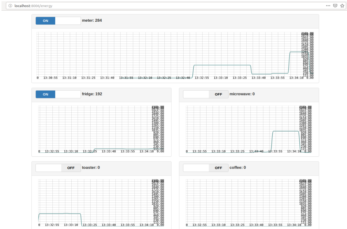
Figure 14. Energy consumption from the smart plugs.
