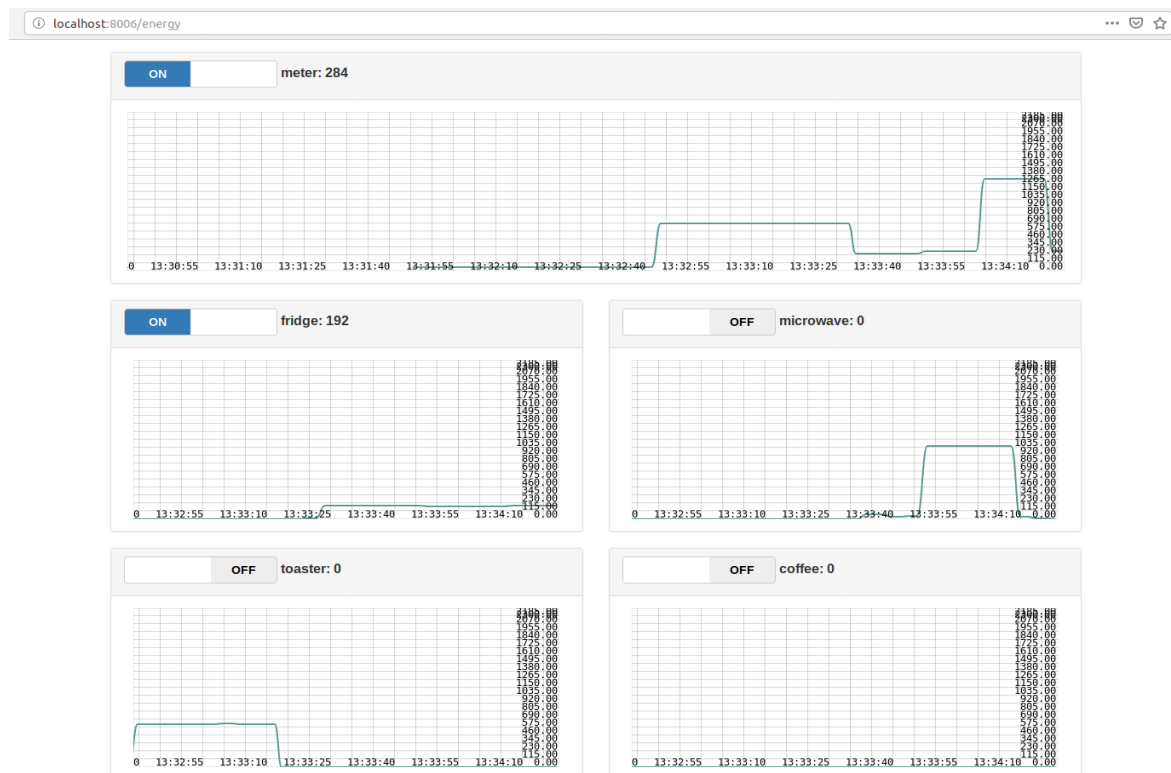
Figure 14. Energy consumption from the smart plugs.
