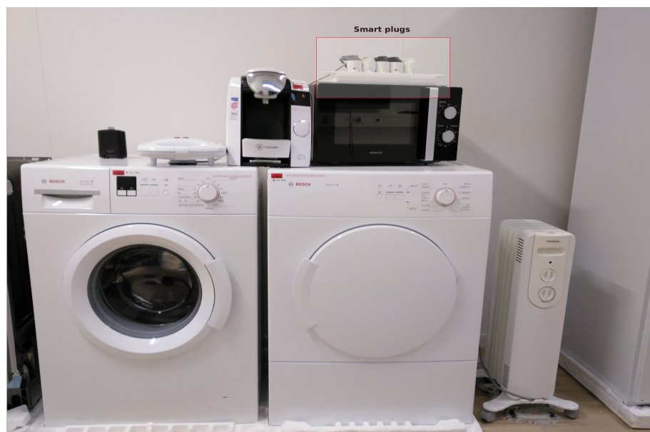
Figure 9. Smart home appliances attached to smart plugs.
