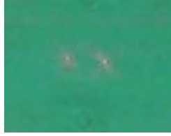
Fig. 3. Two movable array of traps rotating two beads in a 10.5\ \mu\text{m} circle with maximum speed of 35\ \mu\text{ms}^{-1} . Movie at: http://www.cosmic.ed.ac.uk/movies/tweezers/holographic/fast_speed.avi
