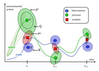
FIG. 3. Sketch of sequential data assimilation algorithms in the observation space where  $\mathbf{H}$  is omitted for simplicity reasons. The ellipses represent the error covariances computed from the Kalman-based equations, i.e. the forecast  $\mathbf{P}^f$  and analysis  $\mathbf{P}^a$ , as well as the model error  $\mathbf{Q}$  and observation error  $\mathbf{R}$ , unknown entries of the state-space model in Eqs. (1-2). This is a modified figure based on Fig. 1 from Carrassi et al. (2018).
