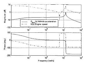
Fig. 2. Bode diagram of G(s) function engine speed and  $G_{acc}(s)$  function acceleration
