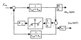
Fig. 1. Simplified model of powertrain
