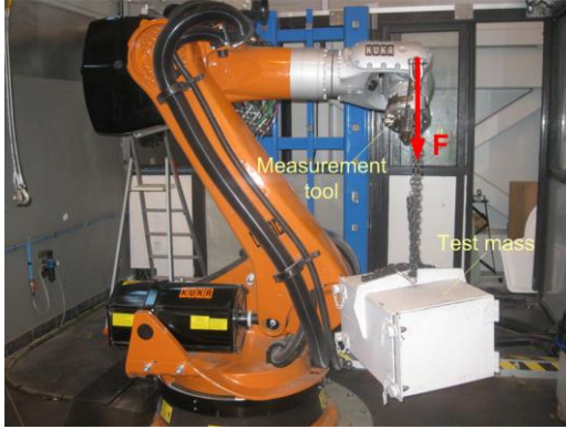
Figure 1. Experimental setup for the elastostatic calibration
