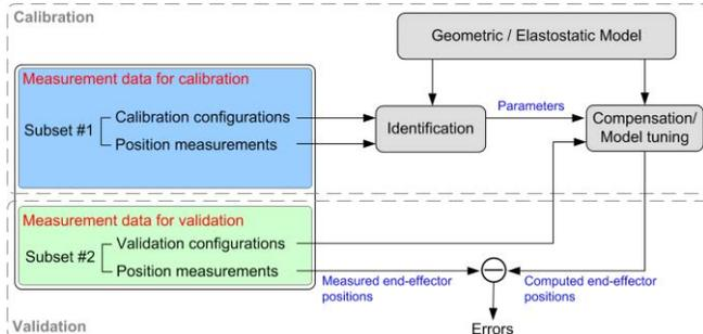
Figure 6. Validation scheme for the calibration results
