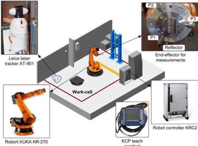
Figure 1. Experimental setup for manipulator geometric calibration
