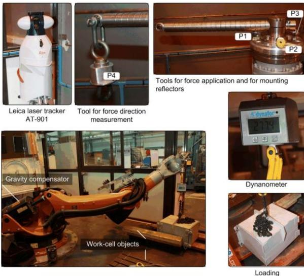
Figure 2. Experimental setup for manipulator elastostatic calibration
