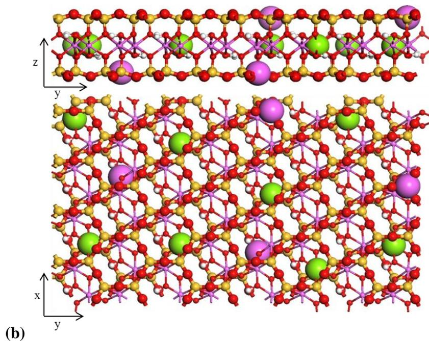
**Figure 1.** Side and top views of the upper (a) and lower (b) TOT layers of the most disordered clay model *RanTO*. The color code is: Si (yellow), Al (pink), Mg (green), O (red), and H (white). Similar structures corresponding to the models *Uni* and *RanO* are provided in the Supporting Information.
