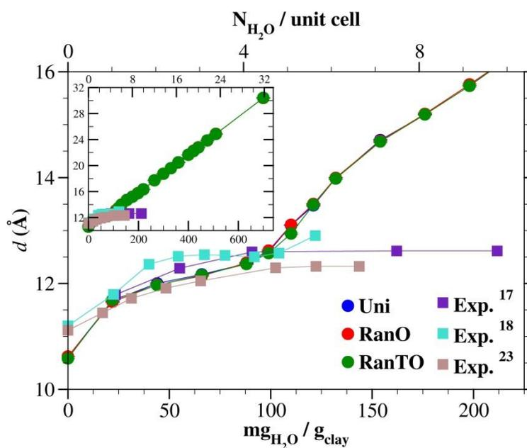
**Figure 4.** Swelling curves of Cs-montmorillonite simulated with three new clay models *Uni* (blue), *RanO* (red), *RanTO* (green). Available experimental data are shown for comparison. The error bars for the simulated values, calculated with a 95% confidence interval, are within the size of the symbols.
