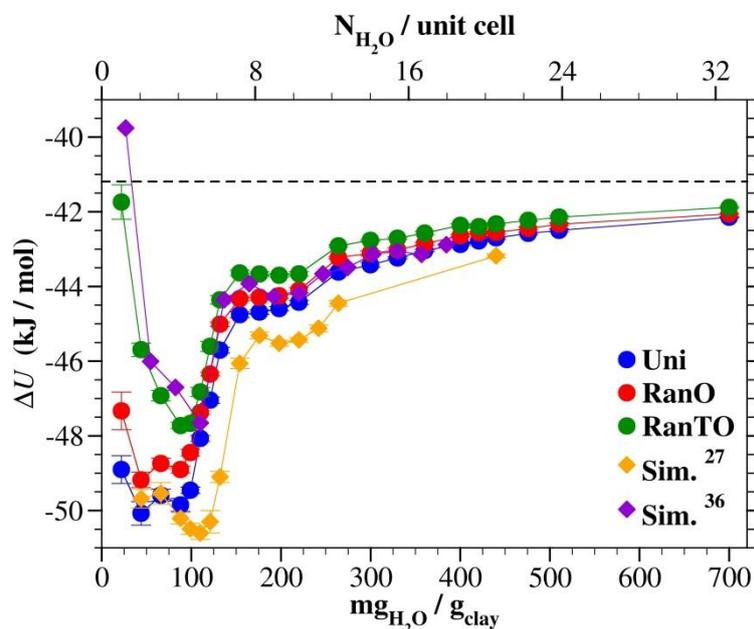
**Figure 5.** Hydration energy curves for Cs-montmorillonite simulated with the three new clay models and their comparison with previous simulations. The error bars are shown with a 95% confidence interval.
