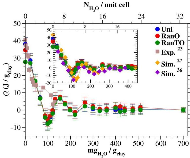
**Figure 6.** Immersion energy curves simulated for the three new Cs-montmorillonite models, and their comparison with experimental data and previous simulations. The error bars are shown with a 95% confidence interval.
