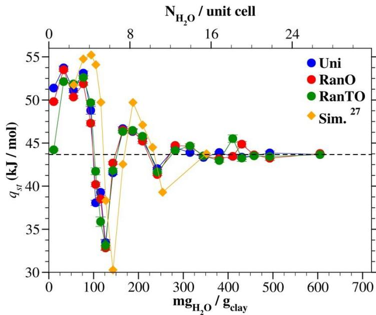
**Figure 7.** Isothermic heat of adsorption simulated for the three new Cs-montmorillonite models. The error bars are shown with a 95% confidence interval.
