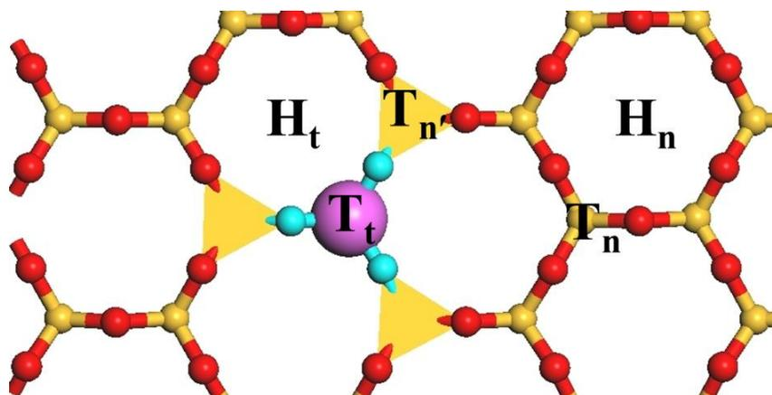
**Figure 9.** Identification of different binding sites on the clay surface: “normal” hexagonal site without substitution ( $H_n$ ), hexagonal site adjacent to tetrahedral substitution ( $H_t$ ), “normal” triangular site without substitution ( $T_n$ ), substituted triangular site ( $T_t$ ), and triangular site adjacent to tetrahedral substitution ( $T_n'$ ).
