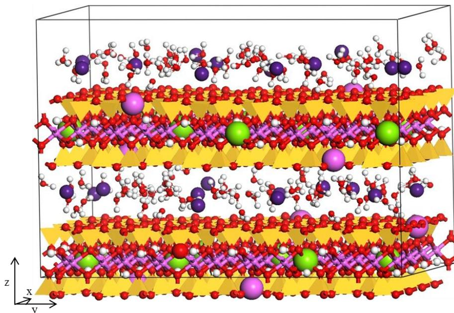
**Figure 3.** Snapshot of one of the simulated Cs-montmorillonite systems with water content corresponding to 6 H<sub>2</sub>O molecules per Cs<sup>+</sup> ion or 5 H<sub>2</sub>O per unit cell (1-layer hydrate).
