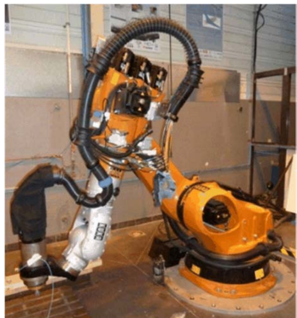
Fig. 6. Industrial robot Kuka KR-270 TM.
