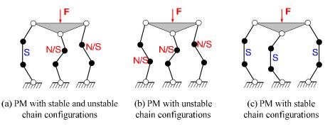
**Figure 2** 2D parallel manipulators with serial chains in stable and unstable configurations
