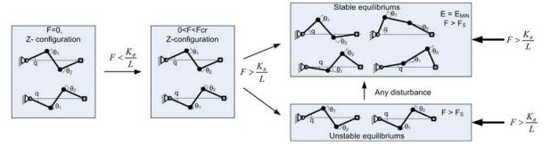
Figure 9 Evolution of the Z-configuration under loading
