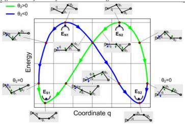
Figure 6 Energy diagram for 3-link serial chain
