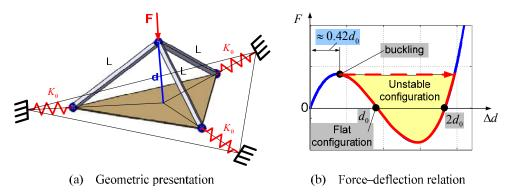
Figure 13 Simplified stiffness model of Orthoglide-type manipulators for near-flat configuration
