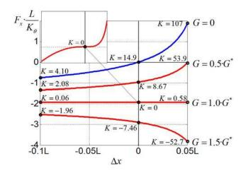
Figure 11 Force-deflections relations for different values of auxiliary loading  $G\left(G^* = 4K_{_{\rm fl}}/L\cdot\sin\alpha_{_{\rm fl}}, K_{_{\rm fl}} = K\cdot K_{_{\rm fl}}/L^2\right)$
