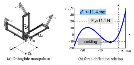
**Figure 12** Force-displacement relations for Orthoglide manipulators (distance to the singularity is 11.4 mm)
